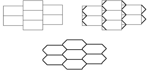
Fig. 2. From rectangle to “almost” quasi-regular hexagon with the same lattice tiling.
